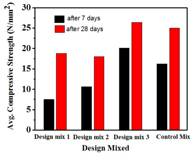
**Figure S1.** Compressive strength of M25 Concrete with various design mix
