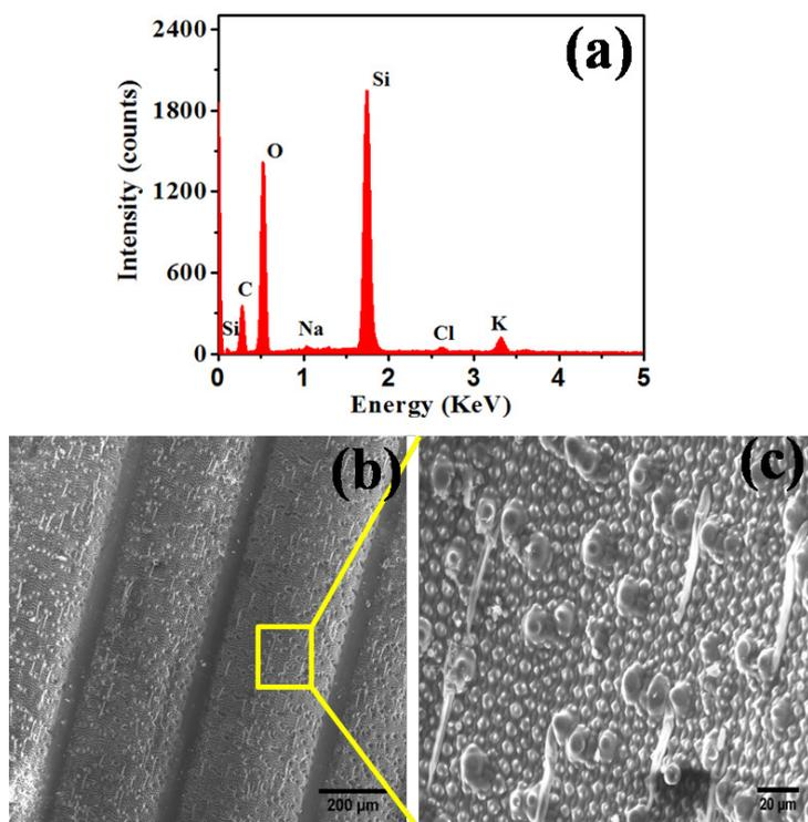
**Figure 2.** (a) EDS analysis, (b-c) SEM morphology of the dry rice straw
