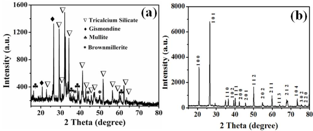
Figure 6. PXRD analysis of (a) Ordinary Portland cement, and (b) commercially available sand
