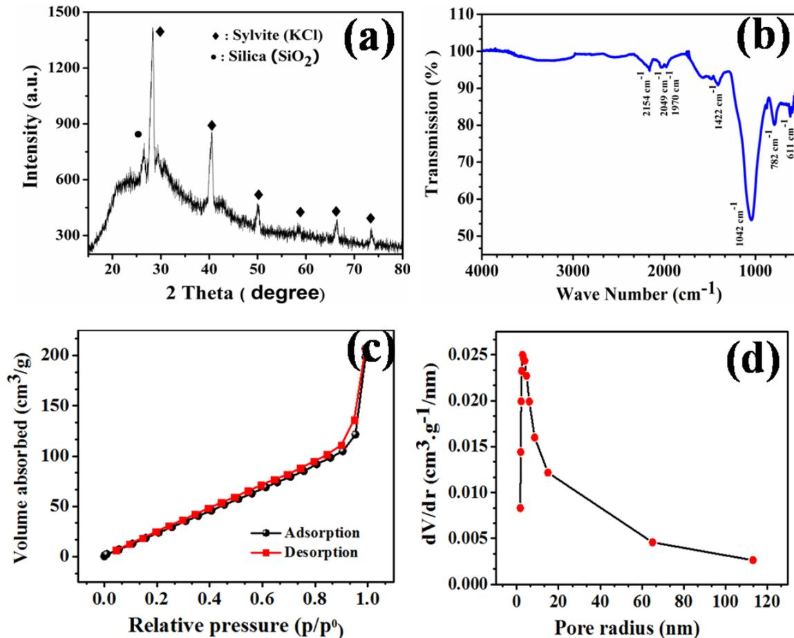
**Figure 4.** Characterization of rice stubble ash obtained after burning of rice straw (a) PXRD; (b) FTIR; (c) BET surface area and (d) pore size distribution
