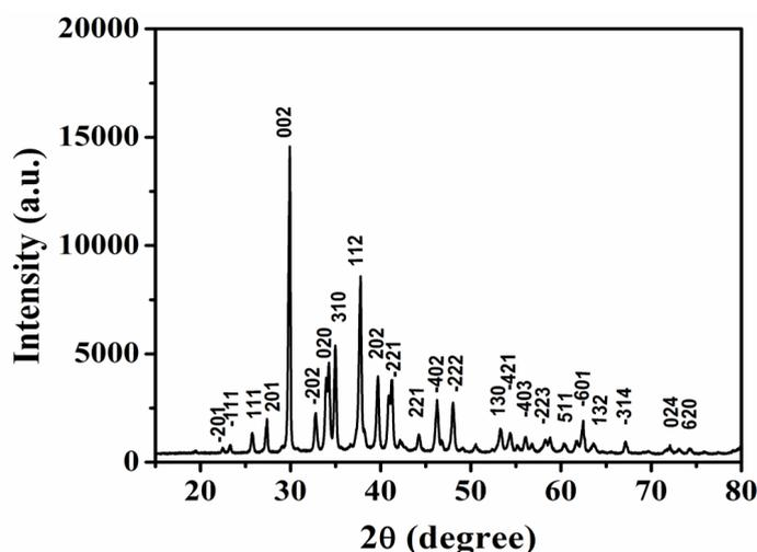
**Figure 3.** Powder X-ray diffraction patterns of sodium carbonate (Na<sub>2</sub>CO<sub>3</sub>)
