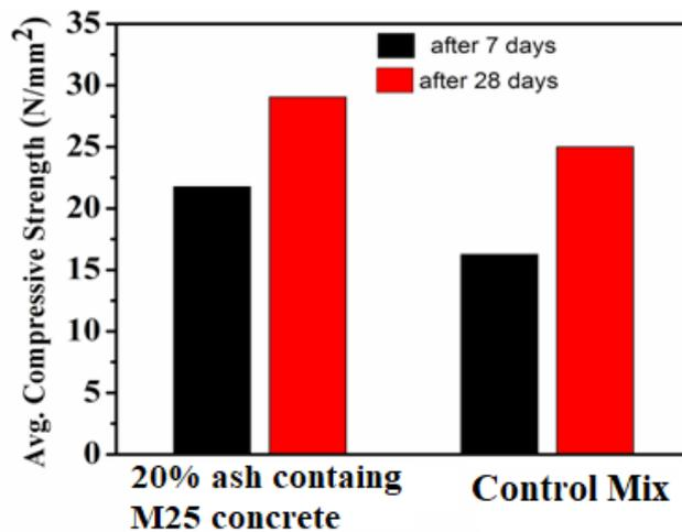
Figure 7. Compressive strength of M25 Concrete with 20% ash
