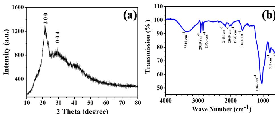
**Figure 1.** Characterization of dry rice straw (a) PXRD analysis; (b) FTIR spectra
