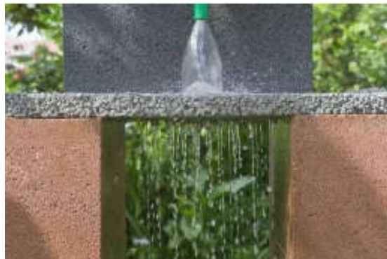
Figure 1 Application of permeable concrete in landscape
