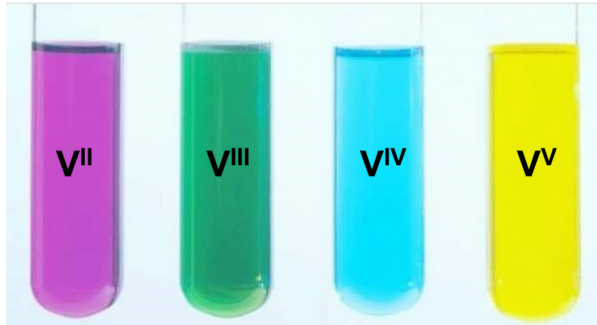
Figure 6. Solution containing vanadium at different oxidation states. From left to right, V V , V IV , V III , V II . Source: © Periodic TABLE Elements
