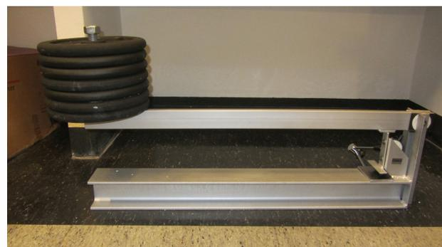
The test press had a support arm formed by a rectangular tube 60.20.1.5 with a total weight of 2.17 kp. The support pivot for the weights was a Ø25 tube with a weight of 0.285 kp, so the total reaction transmitted to the HDPE specimen was 7235.9 N.
