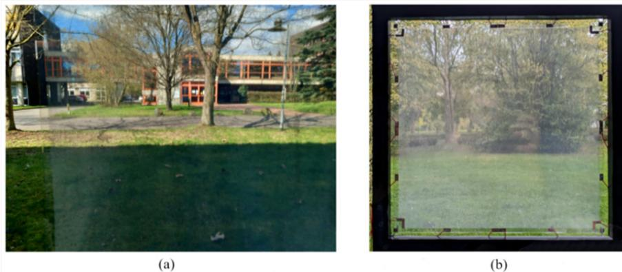
**Figure 6.** Images of a (30×30) cm<sup>2</sup> sample: (a) View through a MEMS micromirror array after fabrication. (b) Window module (double insulation glazing, argon, spacers, butyl sealing) with integrated MEMS micromirror array. The mirror status is partially closed. Contacts for subfield addressing are visible (2×2 subfields).
