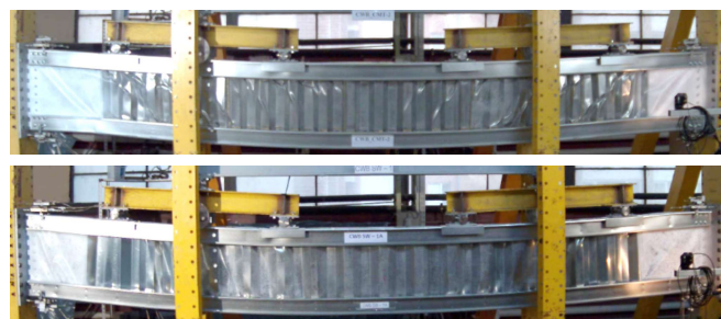
Figure 10. Deformed shape of the CWB after testing a) SW1, b) CMT2
